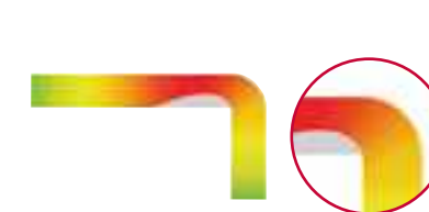
Typical airflow through a standard bend
